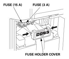
5. Install the fuse holder cover and the battery maintenance cover in the reverse order of removal (see page 64).
