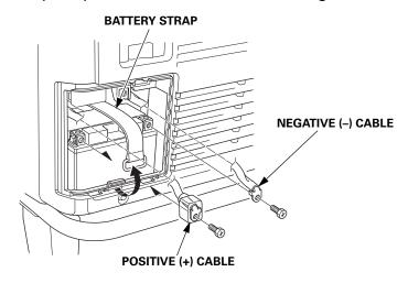
5. Remove the battery from the battery tray.
