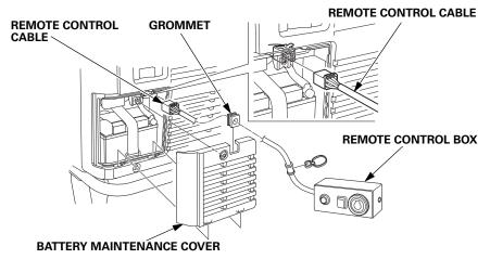
7. To avoid accidentally unplugging the remote control cable, secure the cable to the generator frame with a cable tie as shown.
