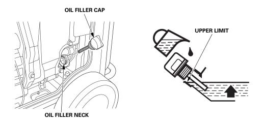
The Oil Alert system will automatically stop the engine before the oil level falls below safe limits. However, to avoid the inconvenience of an unexpected shutdown, check the oil level regularly.
