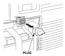
3. View the back of the battery maintenance cover and locate the knockout near the top center of the cover. Carefully remove the knockout.
