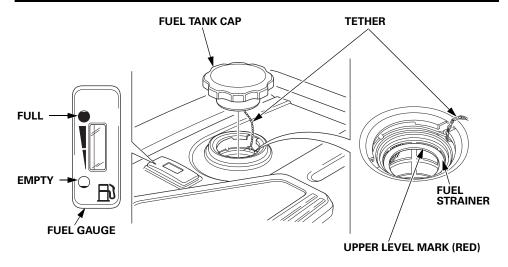
After refueling, reinstall the fuel tank cap securely.
