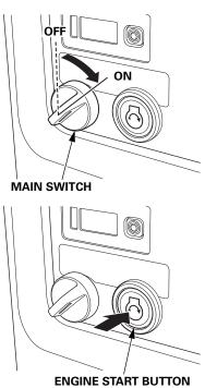
Do not leave the MAIN switch in the ON position when the generator is not operating or the battery will be drained. Turn the MAIN switch to the OFF position when not in use.
