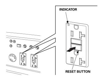
When the RESET button pops out or the green indicator does not light during operation:
