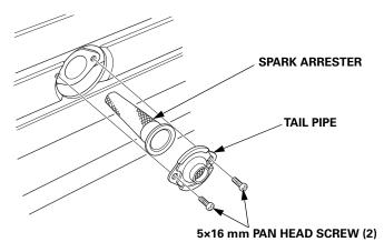
2. Use a brush to remove carbon deposits from the spark arrester screen. Be careful to avoid damaging the screen.
