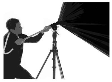
Pivot the reflector to a horizontal position.
