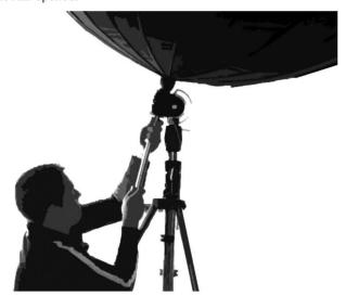
Pull back the extruding bar until the reflector is completely opened.
